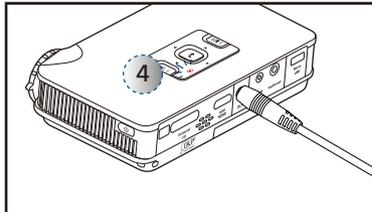
1. Remove protection cap and insert the plug. (①)
