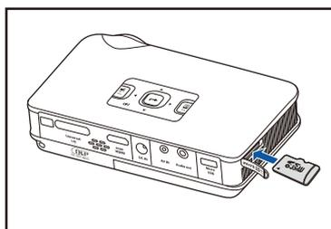
1. Insert a MicroSD card into the slot with the gold contacts facing down.
